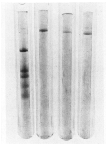
FIGURE 6: 3.0% NaDodSO 4 -polyacrylamide gels. (Left to right) High molecular weight standard [Bio-Rad high molecular weight protein standards (top to bottom): myosin (200 000), \beta -galactosidase (116 250), phosphorylase B (92 500), bovine serum albumin (66 200), and ovalbumin (45 000)]; LDL; NaDC-solubilized apoB; DMPC:apoB 4:1 w/w isolated by density gradient ultracentrifugation and prepared at a ratio of 1:1 w/w.
